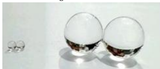
FIGURE 2 Form and size of gel bead before (A) and after (B) swelling
