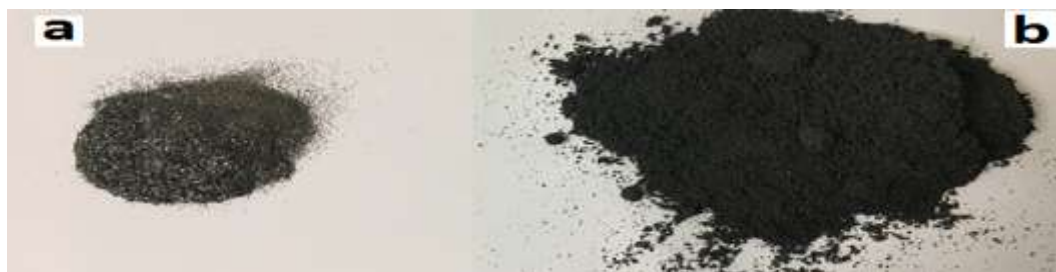
Figure 2. Natural graphite powder (a) and exfoliated graphite (b)
