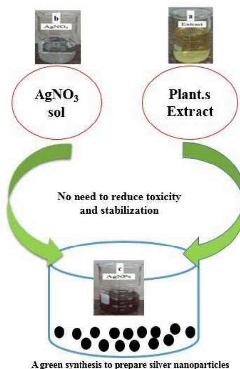
Figure 1. Synthesis of silver NPs by Scropholaria Striate
