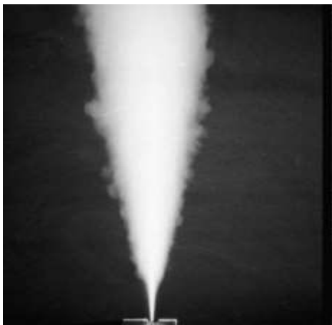
Figure 1. The flow of a high-speed gas jet and spreading it in surrounding [15]
