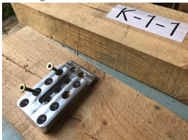
FIGURE 3 Installation of the groove-type plate on the main beam of the joint
