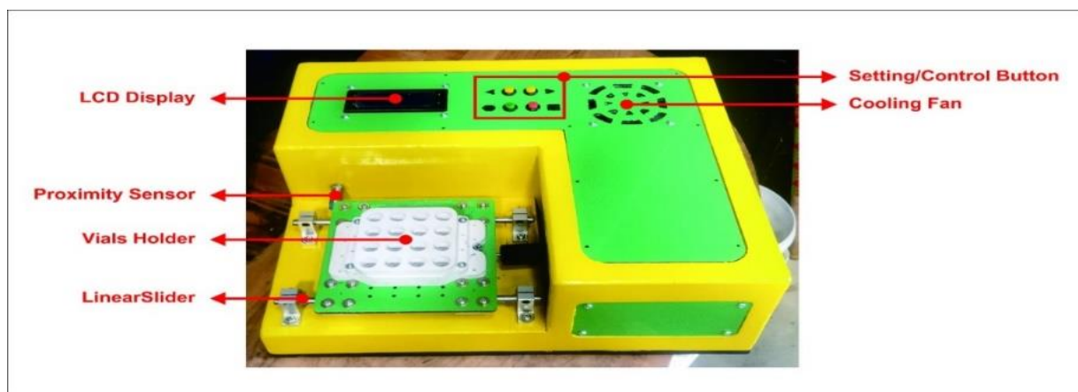
FIGURE 1 Results of the design tool "Blood Tube Shaker Machine"
