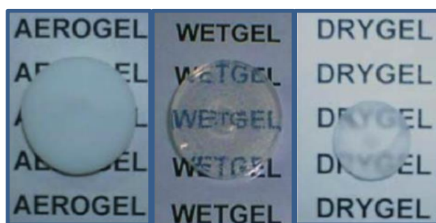
FIGURE 2 a) wet gel, b) dry gel, c) aerogel
